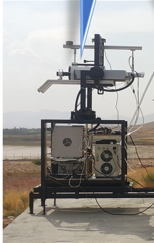
The lidar in Zenith and Horizontal measurement setup
