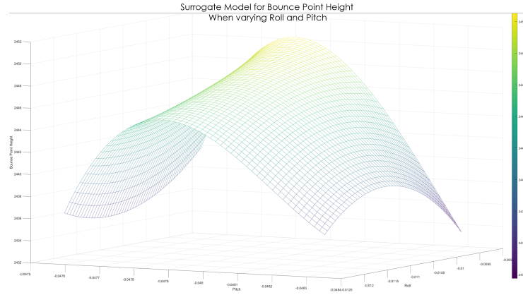
Fig. 3. gPCE model evaluated at a single data point with all variables held constant except roll and pitch, to show bounce point height sensitivity to roll, pitch, and roll+pitch effects. (Roll, pitch ranges kept broad for illustrative purposes.)
