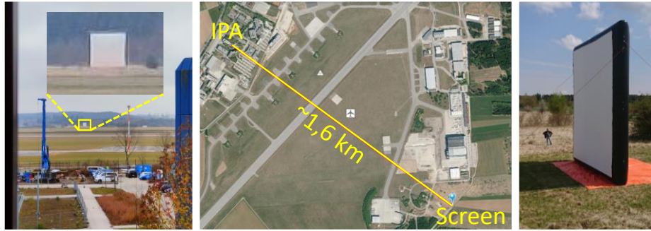
Fig. 4. From left to right: view from the laboratory window, location of the test range in Oberpfaffenhofen and 7x7m inflatable reflective screen ready for use.
